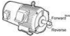
Figure 3.2 Rotational Direction of Motor
