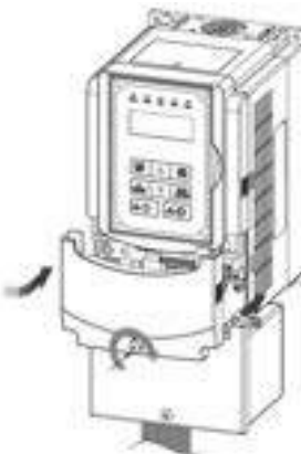
Step 5: Make connections and place filter cover back
